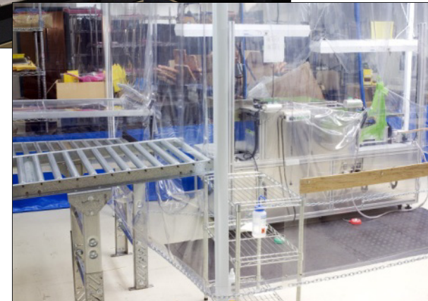
High-Speed Laminator in Class 10 Clean Room
