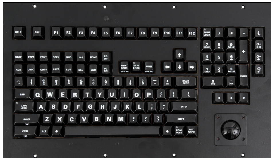
Panel mount 121-key keyboard includes full numeric keypad
